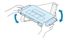
6 Place the toner cartridge on a flat surface, as shown and remove the paper covering on the toner cartridge by removing the tape.
